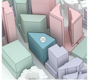
Lowest building height Tower GFA per level 1,956m<sup>2</sup> Tower NLA per level 1,760m<sup>2</sup>
