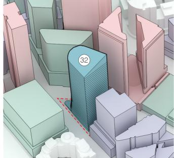
Applicant's proposal Tower GFA per level 1,292m<sup>2</sup> Tower NLA per level 1,221m<sup>2</sup>
